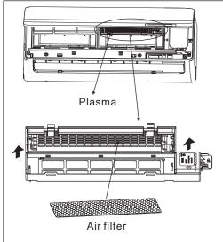
Hold the two parts of Plasma where are marked with 🛧 signal and lift it. Then you can open the cover of the the plasma and remove the filter. (2)
