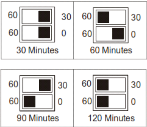
Dipswitch Settings for Selection of Defrost Time
