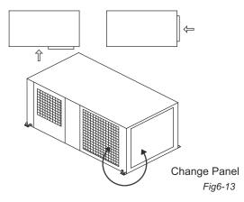
To change air outlet is necessary to interchange panels too. Fan outlet panel is attached to fan structure, which must be mounted as follow.
