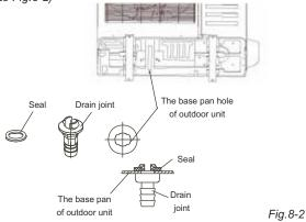
Outdoor unit is equiped with a drain piping. Its position is shown figure below
