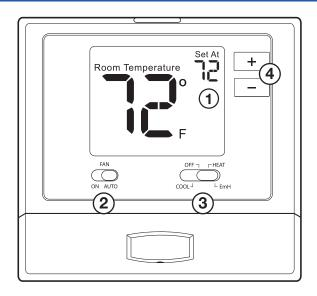
1LCD3System Switch2Fan Switch4Temperature Setpoint Buttons
