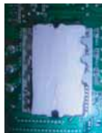
OK : Evenly applied silicon grease.
