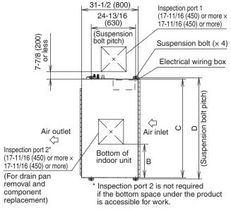
Fig. 3-2 unit: inch (mm)
