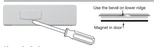
Gently slide a screwdriver into the bottom edge of the badge. Gently turn the screwdriver counter clockwise. The badge is held on by a magnet in the well of the battery door. The badge should pry off easily.
