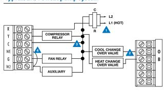
Typical 2H/1C heat pump system with seperate emegency heat
