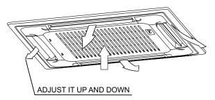
While this function is set, the swing fan of indoor unit runs; otherwise, the swing fan doesn't run. The swing scale of every side is 30°. When the air conditioner isn't in operation (including when "TIMER ON" is set), the SWING button will be disabled.
