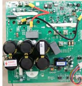
5) Disconnect the connectors and wires connected from PCB and other parts.
