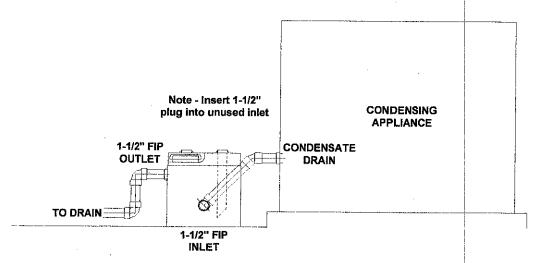
WARNING - "Risk of damage to appliance". Neutralization tank inlet and discharge must be at a <u>lower</u> elevation than the condensate drain from the appliance.
